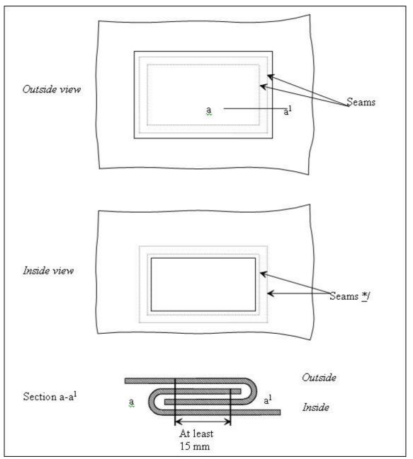
\*Threads visible from the inside shall have a colour different from that of the threads visible from the outside and from that of the sheet.
