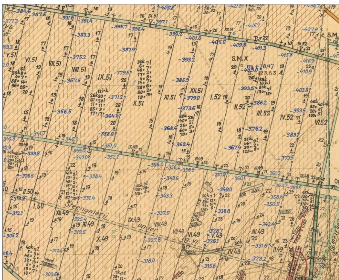
Fig. B 11: Detail of mine map with NAP levels of the coal layer (in blue), tables of excavated coal (k), and shale beds (l)
