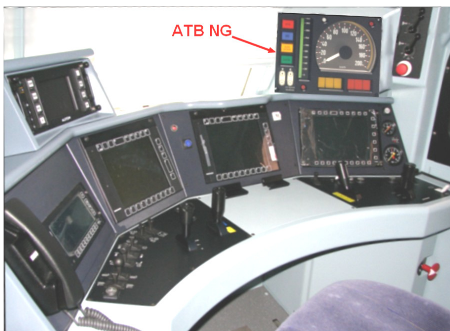
Image 14 - Drivers desk loco class 186 or 189 with ATB-NG cab display
